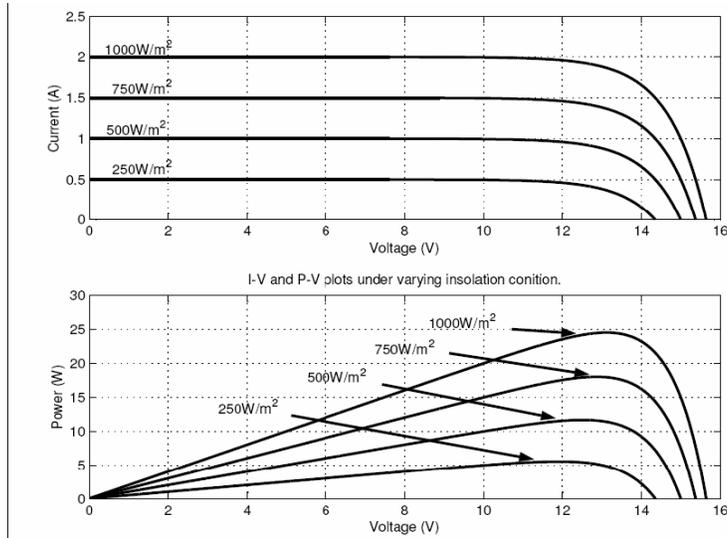
Fig. 6 Changes in the characteristics of the solar pv module due to change in insolation level
