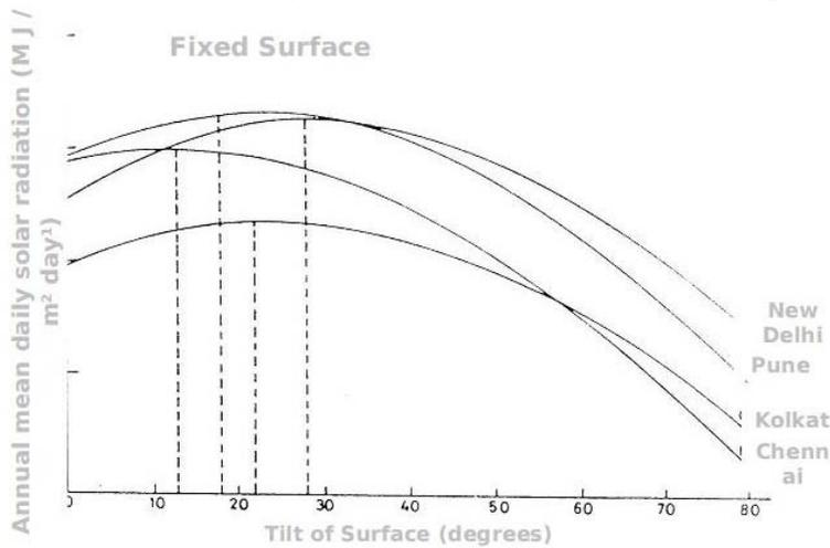
Figure 7: Global radiation at different tilt angle
